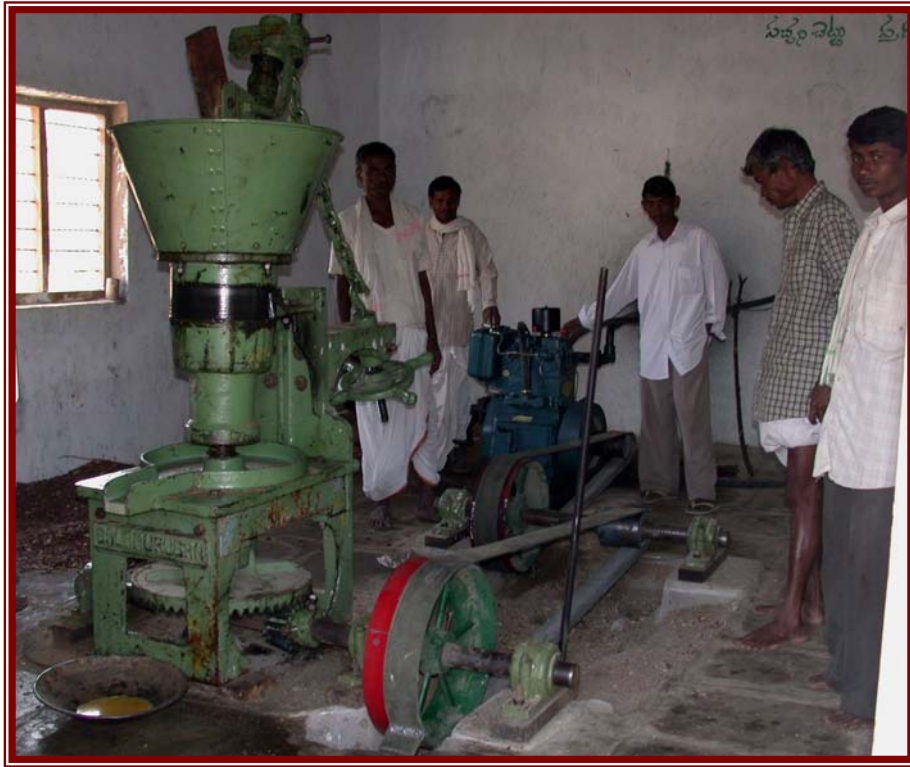
Figure 2. Pongamia oil expeller unit
