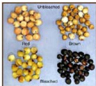
Figure 3. Chlorox bleach test of non-tannin and tannin sorghums.
