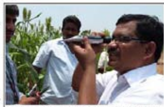
Measuring the sugar content of sweet sorghum stalk with a hand refractometer. Photo: M Gyles, ICRISAT
